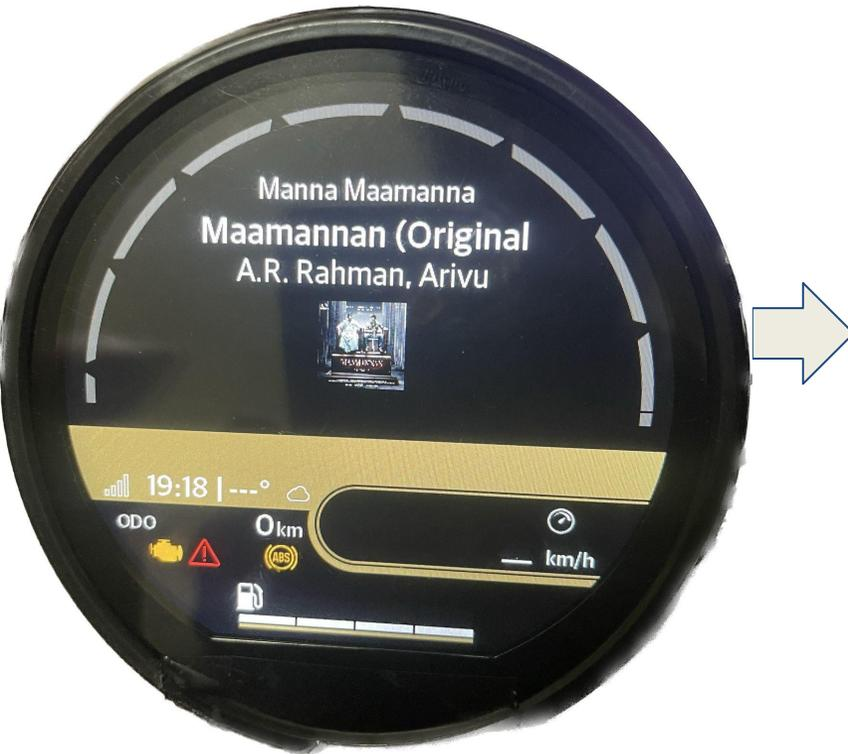
5. Music control should be available for the rider to control, Rider should be able to change the track using the Joystick available at the handle bar
