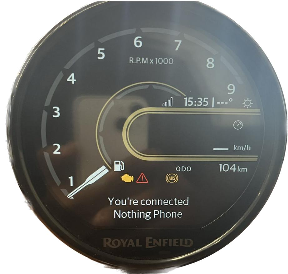
5.1: Cluster when the Device is connected and the Map Navigation is not started
