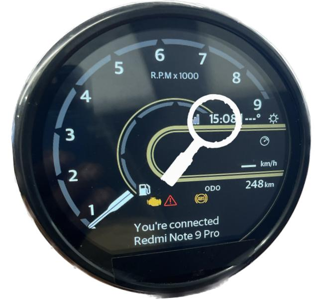
3.1 Connected device information is displayed when the Cluster is connected
